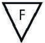
The symbol indicates the suitability of fixtures to be mounted directly on normally inflammable surfaces. Fixtures without the above symbol are only suitable for installation on non-flammable surfaces.
