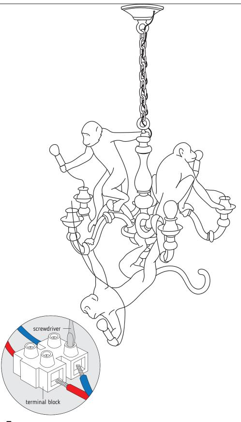
**3.** Connect the wires using a terminal block: red cable connects with L, blue cable connects with N
