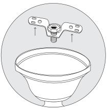
**1.** Unscrew the bracket from the semi-sphere
