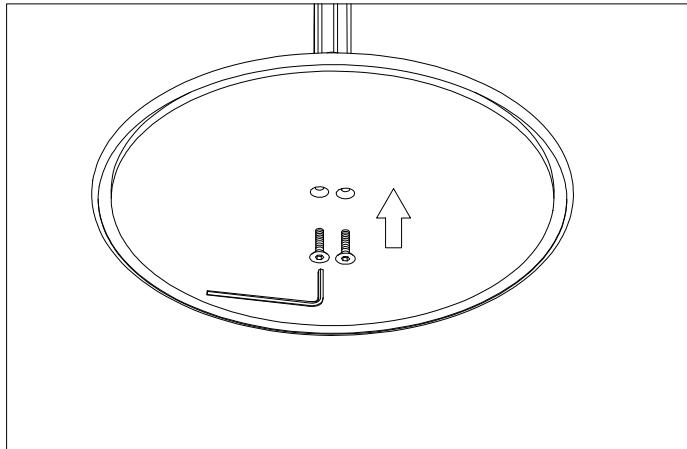
2 Fix the base to the stem by using the 2 screws in equipment (Kit)
