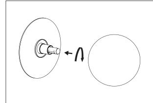
Carefully place the glass globe over the light bulb. Turn clockwise to attach the glass
