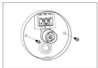
Mount the back part of the lamp to the wall or ceiling with screws.
