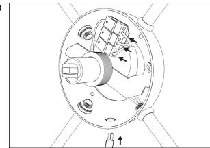
Lead the power cable in through the back or bottom of the where the cable connector resides.
