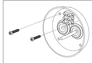
Mount the wall cup to the wall with screws.
