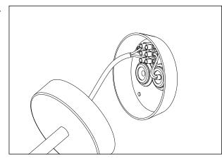
Connect the wire-ends from the lamp to the cable connector.
