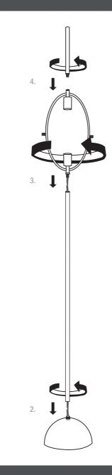
Mount the trestle on the lamppost and tighten it in the direction indicated.
