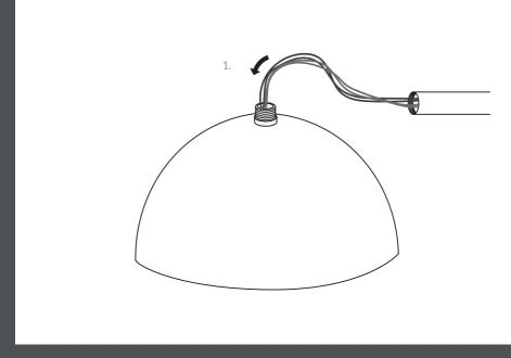
Route the wires down into the base so they are out of the way.
