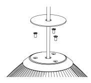
Assemble the top part by placing the hat (4a) on top of the shade and attach with the screw (4b). Make sure it's properly tightened.
