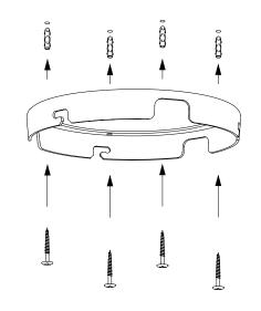
Drill holes. make sure to use plugs and screws matching the ceiling material. Now mount the ceiling fitting.
