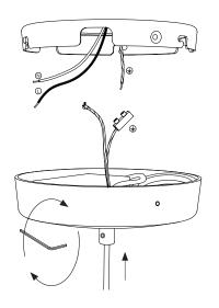
3. Use two fingers to adjust the length of the cord by pushing up or downwards. Roll up the excess cord and place it inside the canopy. Use the Large Hex-key included to secure it.  Connect the earth cable with the loop to the ceiling frame, and the earth cable with the terminal to the earth cable coming out of the ceiling.
