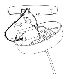
5. To install cables, remove the green cap, then install both cables, natural (N) and live (L). Mount the cap back on the driver.
