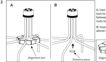
A: Use the cardboard alignment tool to ensure even distance between the arms. Tighten the nuts to lock the arms in place.
