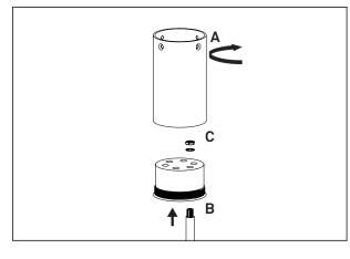
A: Disassemble canopy by unscrewing the tube around the canopy.
