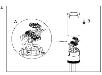
A: Shorten the pendant cables and connect the cables in the 2 pole cable terminals.
