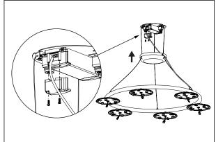
Shorten the lamp cable if necessary and connect it to the secondary (low voltage) side of the driver.
