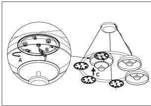
A: Place glass on lamp base and turn the three locks to hold it in place.
