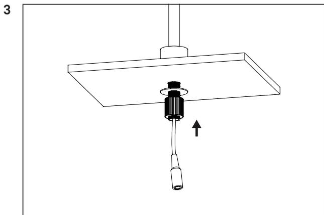
Place the washer and the hand screw over the cable and tighten against the mounting surface.
