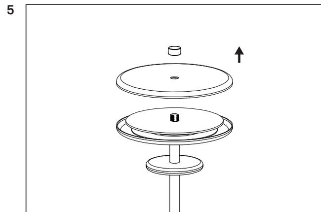
Unscrew the finger screw on top of the lamp and remove the cover plate.
