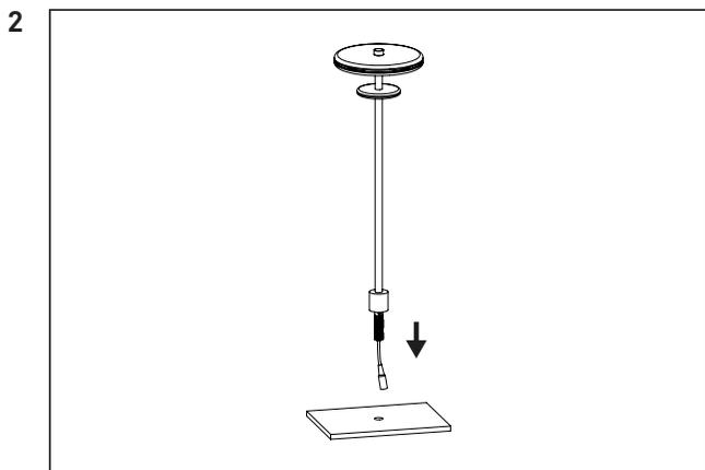
Place the threaded part in the bottom of the lamp into the hole.
