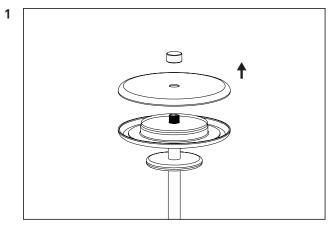
Unscrew the finger screw on top and remove the cover plate.
