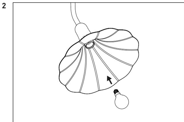
Place an E14 light bulb in the socket. The bulb is NOT included.
