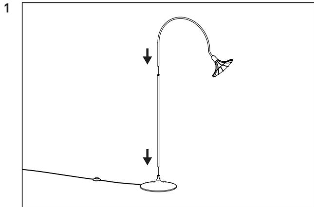
Assemble the lamp by screwing the tube sections together. The excess cable can be pulled out from the bottom.
